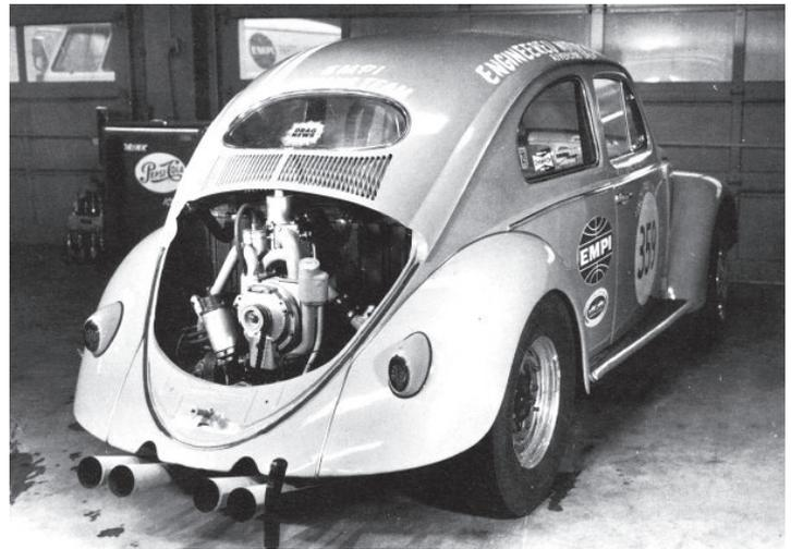
high-quality ported and polished Denzel heads on a 36-bhp-based engine, with Solex 40P11 carbs and velocity stacks from an old Porsche Super 90. It was fitted with light-weight Radar aluminium wheels. This combination was enough to run down into the 13-second bracket. When the BRM wheel made its debut in 1966, the Inch Pincher was one of the first cars to have them.
