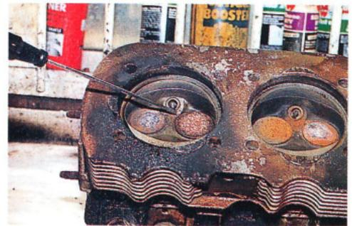
Cracks between valves are alright, but the head is scrap if cracked between the spark plug hole and exhaust valve.
