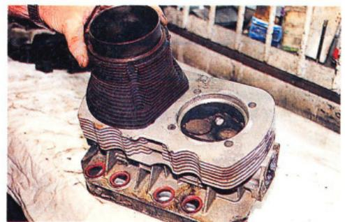
There's no gasket between cylinders and heads. Apply grinding paste and rotate cylinder under its own weight.
