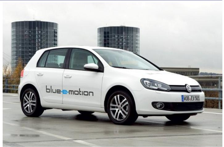
powering the electric motor is stored in a lithium-ion battery bank, with an energy capacity of 26.5 kilowatt-hours.
