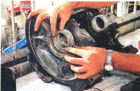
Collar on shell bearing takes up crankshaft thrust. Check there is no play between bearing and journal.
