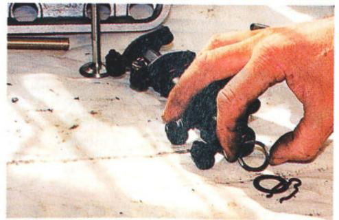
Rocker gear is over-engineered and well lubricated, so should last well. Check spring washers: they can snap.
