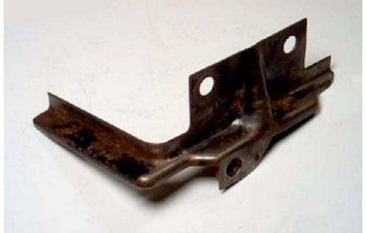
You don't have to remove the fastener to remove the fan shroud, just loosen it. The fastener is usually a slot head machine screw, as for the other tin-ware. (I like to use bolts instead of screws.) It should have the large diameter washer plus a warpy washer. It fits in the notch just beside where the air-vane return spring is fastened.
