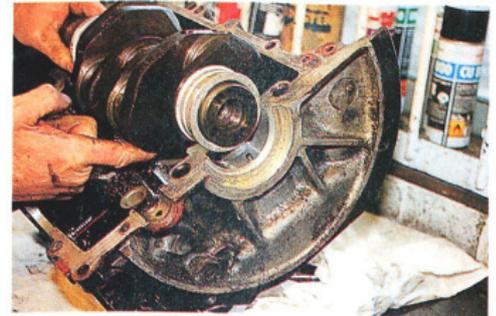
Ensure pegs sit correctly in crankcase holes, and that they locate in bearing shells when you lower the crank.
