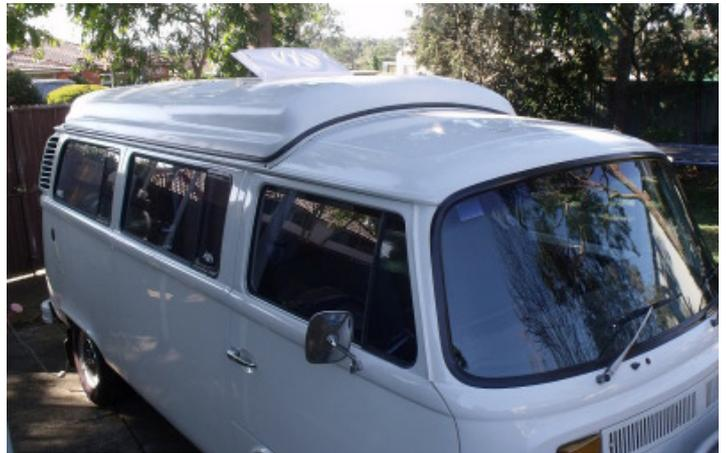
mounting bolts, and another four holes (two on each side) for the support struts. I used my old vent cover as a guide and the new one fit perfectly.
