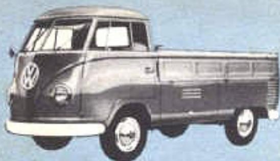
**THE VW PICK-UP** carries a 1764 lb. payload on a 45 sq. ft. load area — plus a weathertight lock-up compartment that provides 23 cu. ft. additional space. Sides and back can be lowered for easy loading from all sides.
