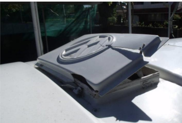
Fortunately it's only held on to the roof by two small hinges and small stainless nuts and bolts, which were OK, and likewise the two support struts with wingnuts. It was a simple matter to unbolt the ruined hatch with an 8mm spanner. But – where to get another one?
