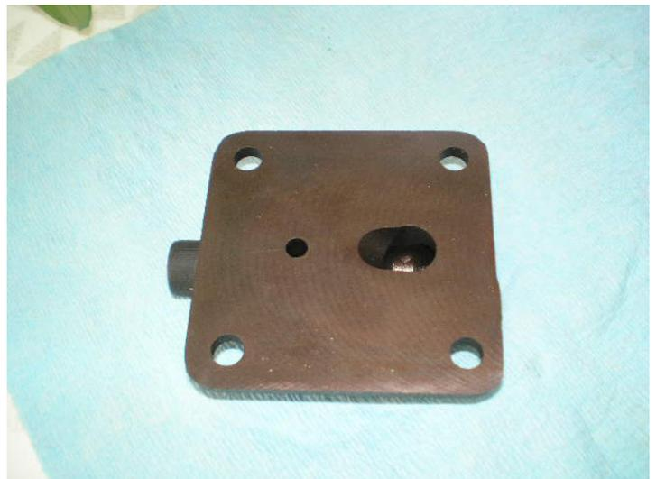
Before using the GB-239 I take it apart, clean it good and break all the edges with a file. The socket-head screw securing the pressure spring goes into the jig and gets drilled for safety wire. The sharp edges of the outlet port are polished smooth then the Blanchard-ground surface is burnished on a surface plate using #600 W&D flooded with WD-40. After a
