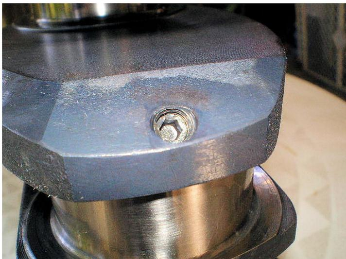
Some of the oil passages on his Chinese stroker are drillings sealed with 4 mm socket-head set-screws. They need to be pulled and the oil passages cleaned then re-installed with Loc-tite and straked. Which he hadn't done. But even as I explained the what and why I had a hunch he wouldn't bother. After all, he's built a lot of engines. And never had any trouble.
