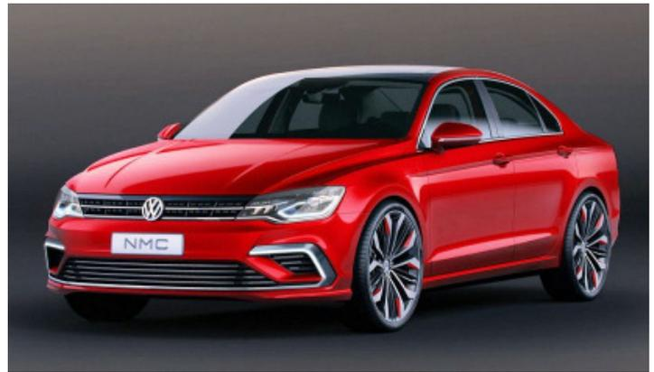
broader than a Passat. The car is built upon the same modular Modular Transverse Matrix (MQB) basis as the current-generation Golf 7 and the similarly sized Audi A3, SEAT Leon and Skoda Octavia.
