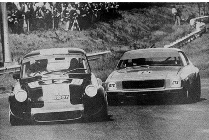
Bryan bought the ex-Warwick Brown McLaren M10B, and most of the mechanical components were fitted in a VW 1600 TL Fastback body shell, including the mid-mounted worked 5.0-litre Chevrolet small block engine. The car debuted at the Calder night meeting in January 1974, and quickly became crowd favourite.
