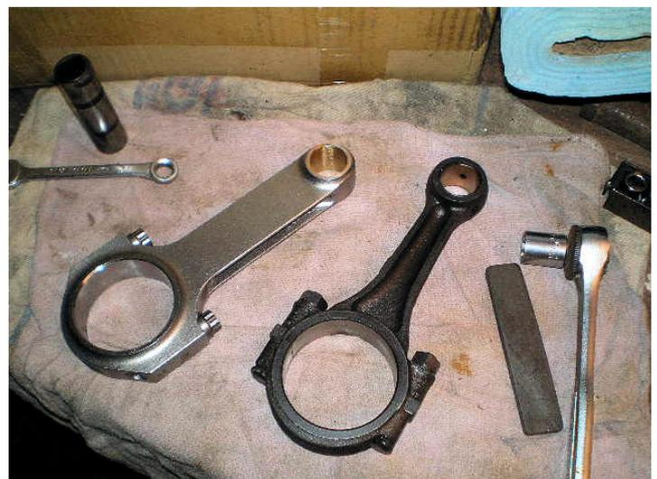
weighs within a tenth of a gram of the other. Of the two heavy rods, one is a tad less than two grams out, the other just over four. Four grams is a lot of grinding, followed by smoothing things up with the belt polisher.
