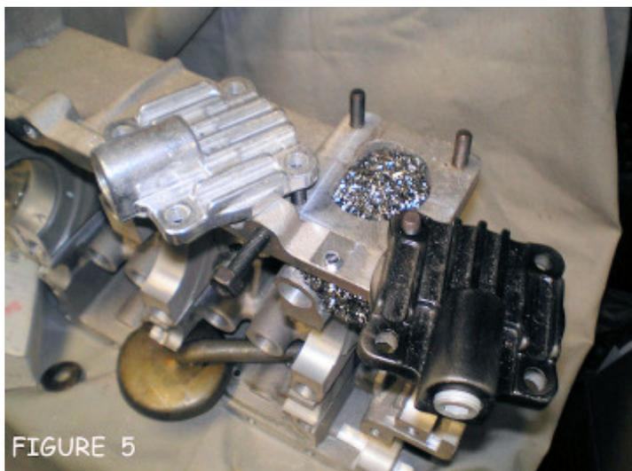
identical, purchased for about \$5 each. The one on the left is as-received, the one on the right has been bead-blasted then treated with a thermal dispersant. (Tech Line's 'TLTD').
