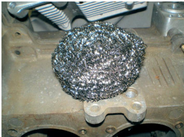
Every crankcase has to breathe. You gotta provide some place for air to flow in and someplace for it to flow out. If your engine's running hot a lot of oil vapour will be mixed with the out-flow. If you don't do something about it, you'll blow it overboard. Which is less of a problem running the Baja than it is flying from here to there. Running the Baja, you can pull over and park.
