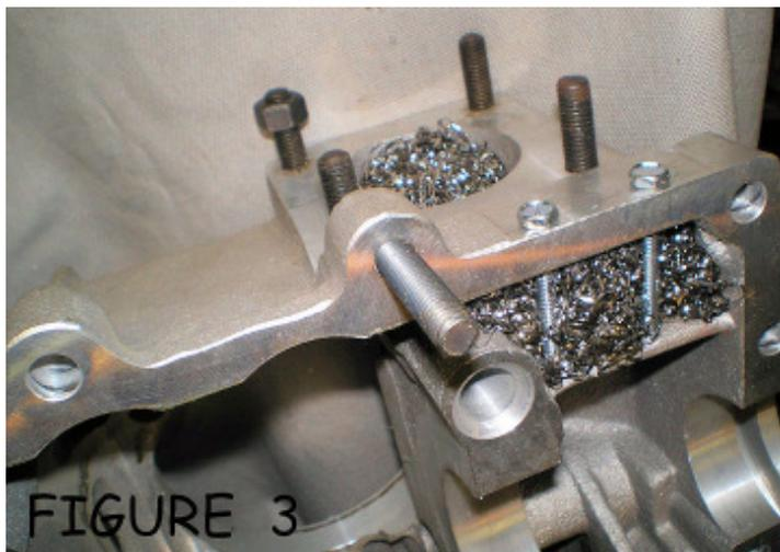
You want the mesh to pretty much fill the D-shaped hole for the dynamo tower but not to bulge above it. That will allow you to use an inexpensive oil pump cover as your outlet. Nor do you want it hanging out the bottom. This is the cam-gear gallery and the last thing you need is to have your mesh get sucked into the gear train.
