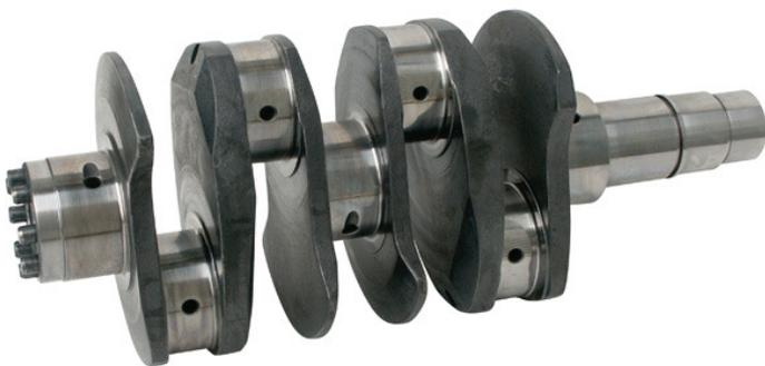
The first crank upgrade above the counterweighted 69 mm crank is the 'Stroker' crank. 'Stroker' refers to any crankshaft with a stroke longer than stock (which in the case of Type 1 engines is 69 mm). This gives more 'leverage'. The driveability and torque of a stroker engine has to be experienced to be believed! A stroked crankshaft allows the
