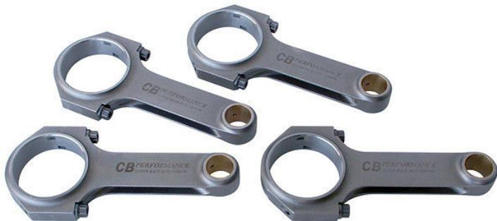
angle is increased. 78 mm is the maximum that the stock rod can withstand; beyond that the bolts will fail. Longer crankshaft strokes require a longer connecting rod, and/or a stronger or a better-designed rod connection system. This is exactly what 4340 Chrome-moly rods accomplish.
