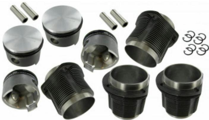
**88 mm:** The next bore size up from stock is the machine-in 88 mm set. These work VERY well, but you are looking at a lot of machining (this costs approx. \$200) for a very small displacement increase! If you're going to go to that work or expense, you should opt for the larger piston set. However, 88s are very good for Buses and Type 3 engines, since these engines run hotter than Beetles, Ghias, or buggies/rails.
