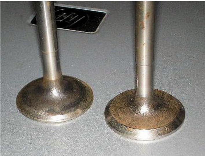
VW Intake Valve, most Type I engines, 1967 and later.
