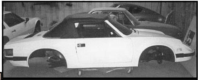
*The Puma "kit" sold in the U.S. required the owner to install front suspension, engine, transaxle, wheels, tires, and battery.*
