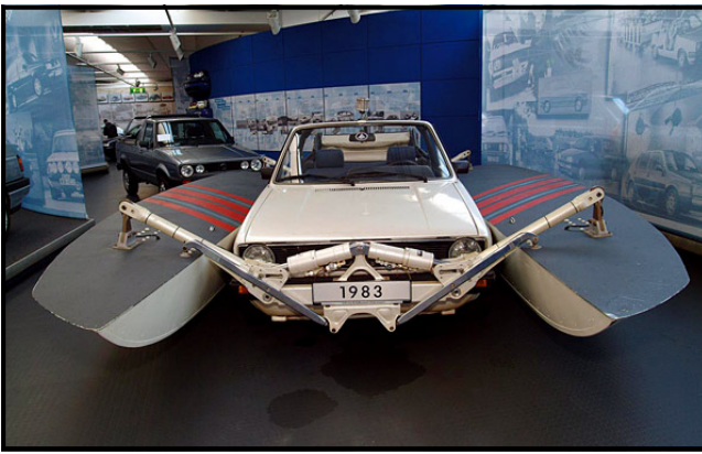
Sea Golf (1983) - The gulf can not only drive but also swim. This Golf Cabriolet with two hydraulically driven swim pontoons was developed and built on the occasion of Golf GTI meeting at the Woerthersee Treffen in 1983.
