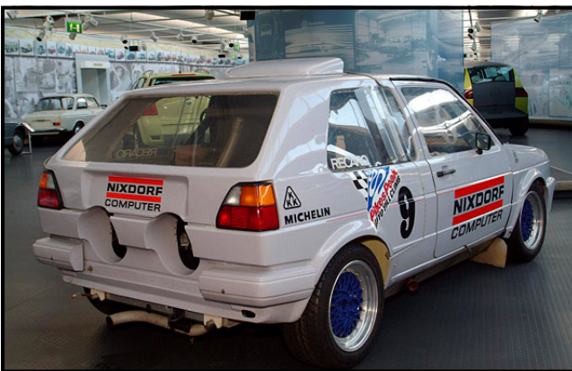
Pikes Peak Golf (1987) - This Golf three was powered by two 326hp engines (front and rear) driving front and rear wheels independently.
