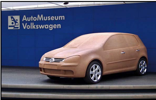
Das Plastilin Design Modell of the Golf V (2003) - This clay model was used in the design process leading up the creation of the final fifth generation Golf design.
