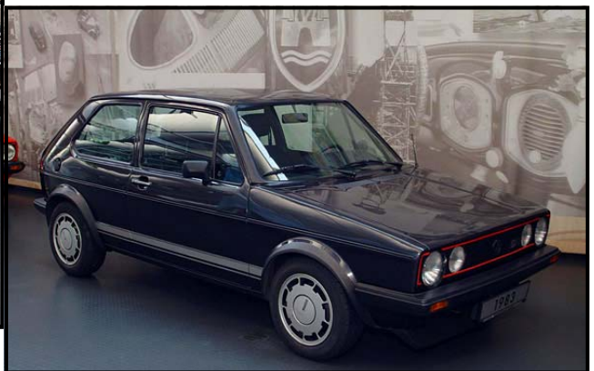
Golf GTI (1983) - This limited edition GTI featured "Pirelli" wheels, special paint, a 112hp powerplant, 5-speed transmission, leather steering wheel, wheel flares in body colour, dual-round headlamps and a "golfball" shift knob. This car featured a 0-60 mph time of 9 seconds.
