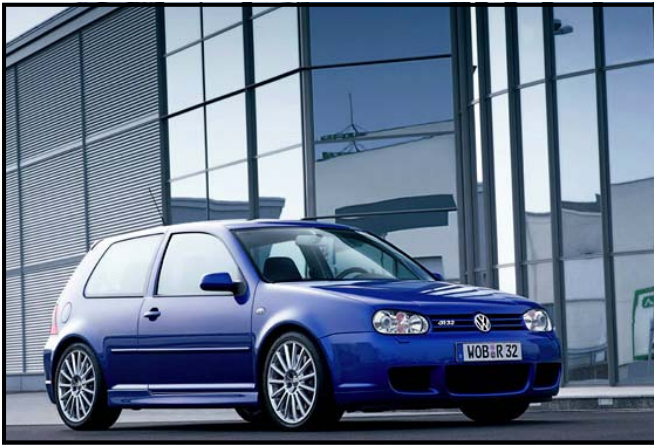
Golf 4 R32 (2002) - Designed to be the ultimate and final version of the fourth generation Golf platform, the R32 features a 241hp 3.2l VR6 engine mated to a six-speed transmission and all-wheel-drive.
