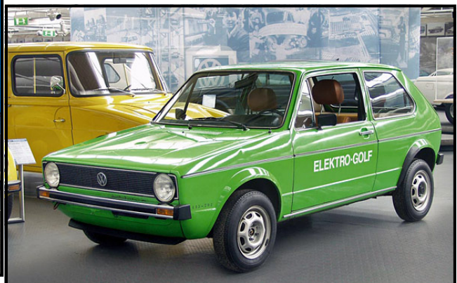
Elektro-Golf (1976) - Designed as a prototype to explore electric drive options this car served for a number of years as a mule for various new electrical technologies.
