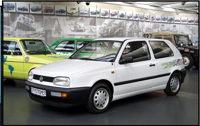
CitySTROMer (1993) - An electric vehicle sporting 16 maintenance-free battery modules, the CitySTROMer was designed to be a zero pollutant vehicle.
