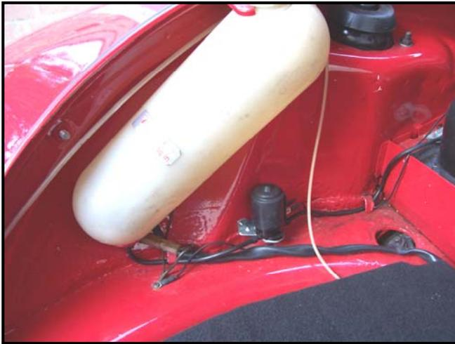
washer motor to one side of the micro switch you have adapted to the back of the original switch, this will require soldering. Then connect another wire from the other terminal of the micro switch back to the 12-volt accessories of the fuse box. That's it for the wiring.
