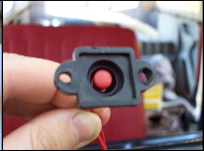
Above is another view of the micro switch screwed into place. The red button is what the insert of the switch presses against.
