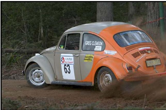
Making sure you are pointing the car in the direction of the apex of the corner pull on the hand brake & de clutch.
