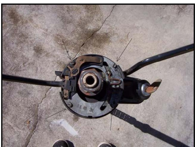
Previous page: A column I had that had been previously removed from a car. When the steering wheel is removed you'll be confronted with this picture. Note: the four screws that hold the assembly into the column.
