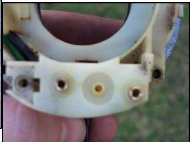
Above: Before the centre hole was drilled out to accommodate the switch.
