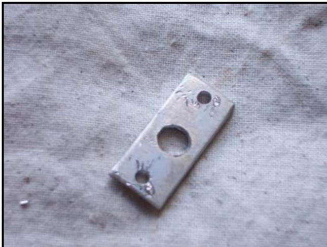
Above: My small aluminium plate drilled and cut to size. See further on in the article how one corner needs to be filed off to allow the switch assembly to fit inside the column assembly.
