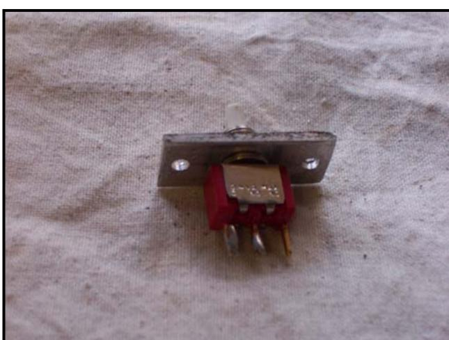
Above: Insert the micro switch into the middle hole of the aluminium and screw the switch up
