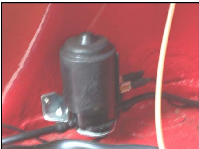
Above: A picture of the washer pump I used. Note the electric motor is above the impellor. This is an important point to remember for installation as described later in the article.
