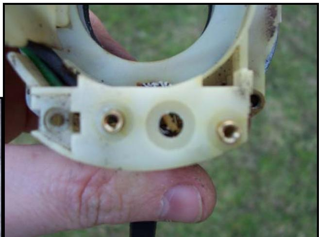
Above: After the hole has been enlarged to accommodate the switch.
