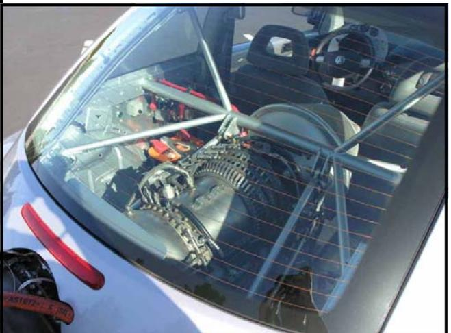
The first thing I did when I got the car was to cut the hole in the back for the engine. Made a fancy jig out of a tripod, a rod, and a lawnmower wheel to mark out the cut and went at it with a pneumatic saw. Then
