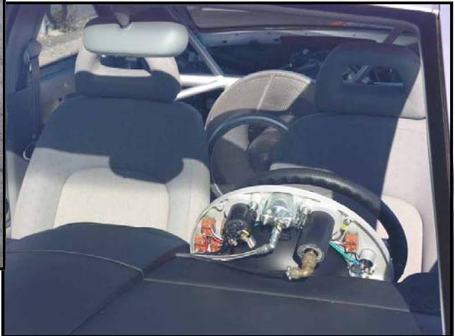
"Jet Under Glass". Air for the jet enters the car through the two side windows and the sunroof. It's a little windy inside but not unbearable.
