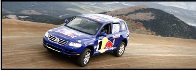
primarily to comply with the safety regulations imposed by the Pikes Peak Race Officials. A roll cage, fire extinguisher, special driver's seat and a five-point racing seatbelt harness were fitted into the interior. Exterior graphics and a set of Nitto Terra Grappler tires were the only other additions to the vehicle.
