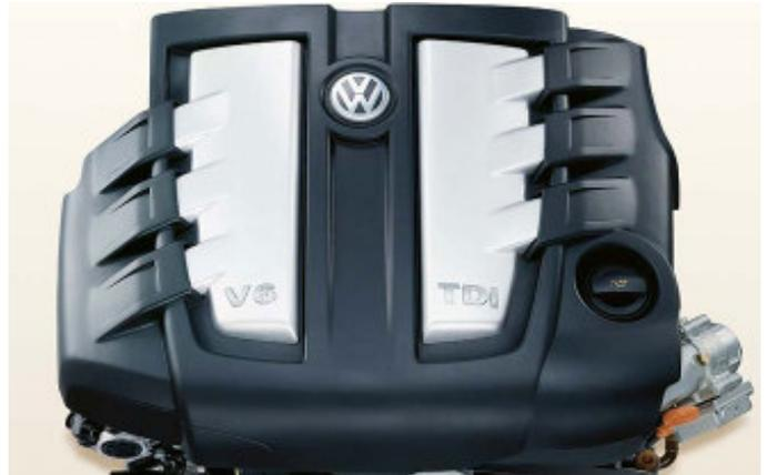
The new V6 TDI engine is 440 mm long, meaning that it is extremely compact. The cylinder crankcase features an angle of 90 degrees and is made from high-strength yet light vermicular or compacted graphite cast iron (CGI). This offers greater strength although it weighs 15 percent less than grey cast iron. The engine weighs only 220 kilograms; its cylinder gap is 90 mm and the compression ratio is 17.5:1.
