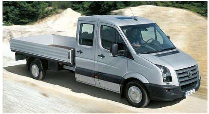
Crafter is designed to supplement the T5 Transporter in higher weight categories. With 3.5 and 5.0-tonne gross weight, the basic models (known as the Crafter 35 and Crafter 50) cover a wide range of uses.
