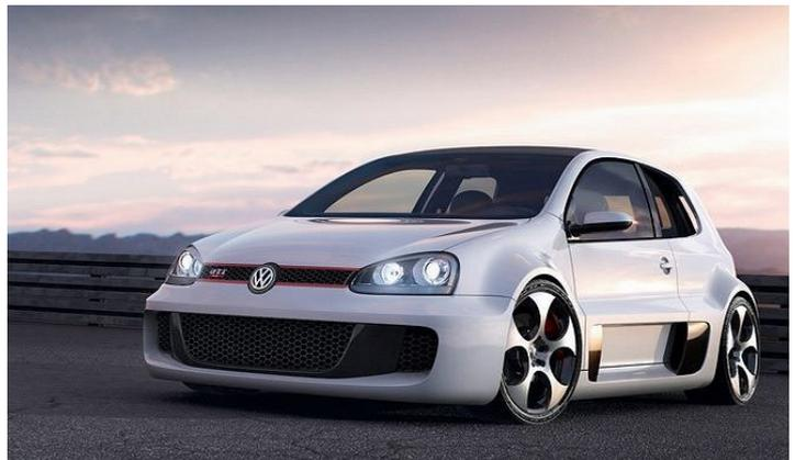
The purposeful new stance is further emphasised by a set of 19-inch wheels styled to mimic the standard wheels fitted to the Golf GTI but, in the case of the GTI W12-650 wrapped in 295-profile tyres to aid traction.
