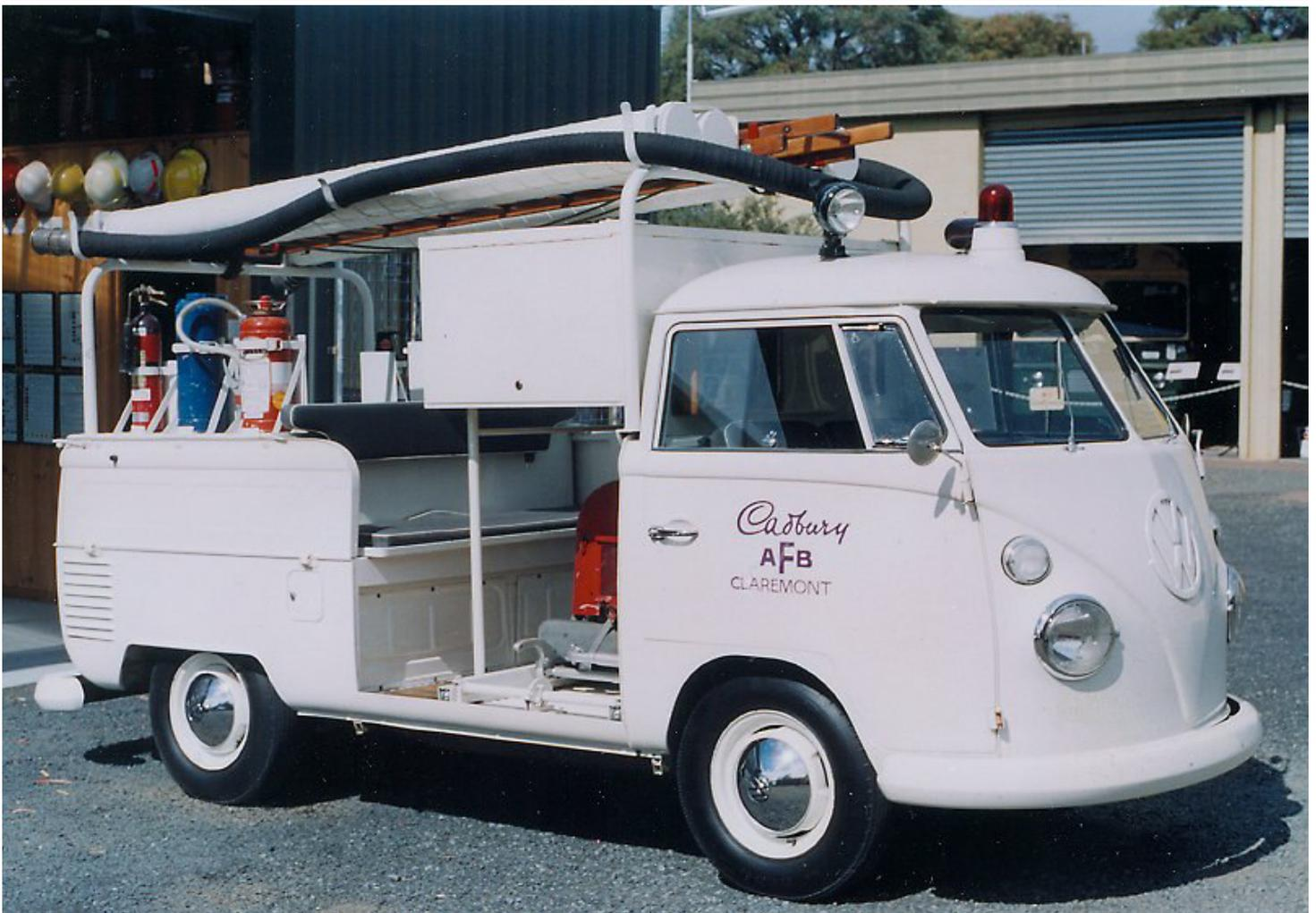
modified to Cadbury's specifications at VW's Clayton facility: mounted midships is a Godiva FWP twin delivery centrifugal pump powered by VW, of course! Also, there's other firefighting equipment such as an extension ladder, portable fire extinguishers and various other gear needed to fight fires of the type that might occur in a chocolate factory. They had electric motors catch fire, fires in flues, hoppers, silos, labs., the cocoa shell plant, bagged sugar store and the incinerator.
