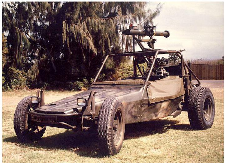
The DPVs had a payload capacity of 680 kg of military gear, and fully laden (2,250 kg) they could accelerate from 0 to 50 km/h in just four seconds, thanks to their powerful engines, light construction and low gearing. They had a top speed of 130 km/h, and with a standard off-road 80-litre fuel tank, had a range of around 380 km in desert conditions. An extra fuel bladder could extend the range to over 1,600 km.
