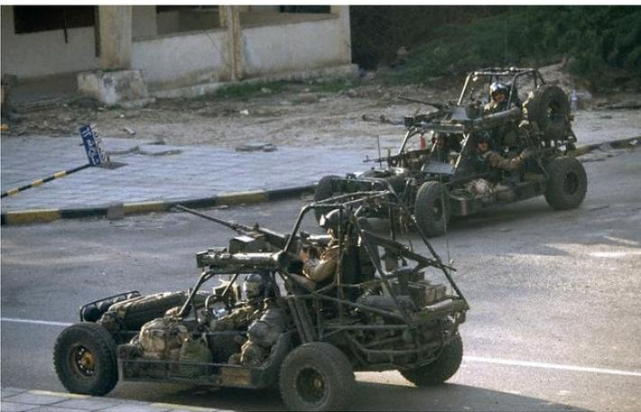
Storm. They were the first air-cooled Volkswagen-powered vehicles used in front-line combat since WW2, but this time they were on the winning side. They really came into their own and were used in a variety of special operations, including commando raids, fast 'attack and run', and the rescue of downed flyers. The first US forces to re-enter Kuwait City were US Navy SEALs in DPVs, and the VWs were seen worldwide on CNN as the US embassy was liberated.
