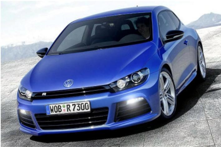
Not unlike the Golf GTI and Audi S3, the Volkswagen Scirocco R is powered by a 2.0-litre turbo 4-cylinder petrol engine that makes use of direct injection to raise the compression ratio, which improves power output. However this engine is tuned to give more power than the GTI engine - in fact it even produces 11 kW more than the 3.2-litre VR6 engine.
