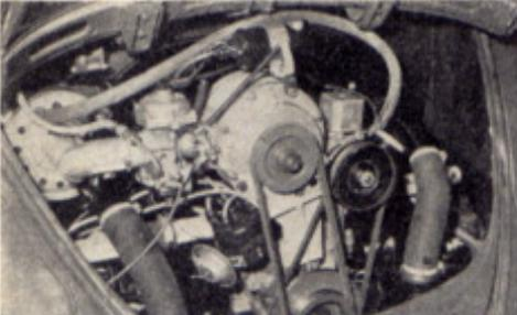
The Shorrock Supercharger fits snugly into the VW engine compartment.
