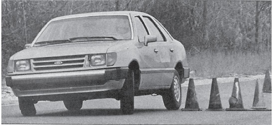
Ford Tempo winds through the maneuverability grid with balance and speed. Note the small amount of body roll the car dodges the last gate.
