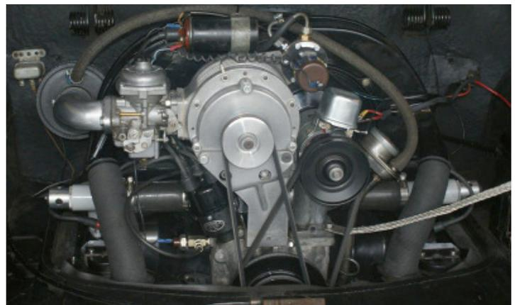
In 1966, Dean Lowry fitted a Shorrock supercharger and SU carburettor to the 1600cc race engine of the famous Inch Pincher race car. On the dyno, the engine produced an astonishing 220 bhp running on straight methanol. With this potent combination on board, Inch Pincher ran a best time of 12.7 sees/106 mph at Carlsbad Raceway. One of the most memorable features of the car at this time was the ear-splitting exhaust note!
