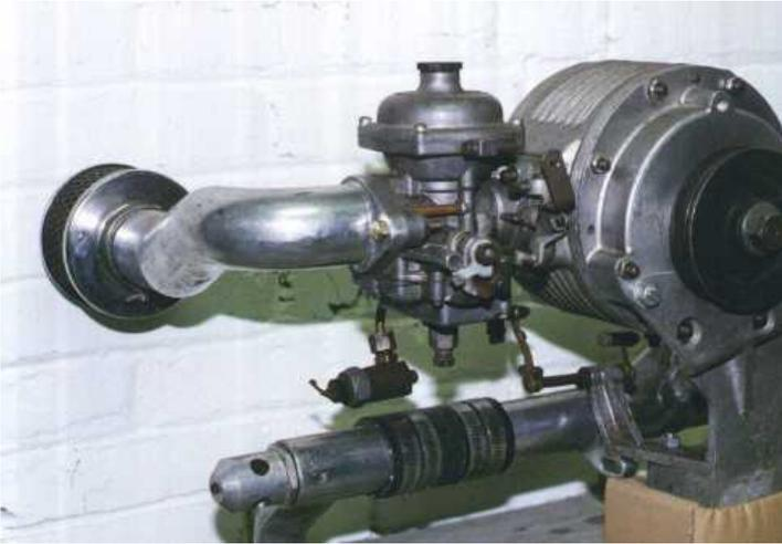
engine and causes less wear and tear on components. It also precludes the need to add oil to the air/fuel mixture to lubricate the vanes, as in the case with the Judson. A separate oil feed is taken from the oil-pressure switch to lubricate the shaft of the Shorrock.
