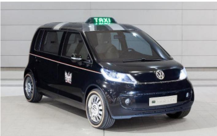
The range of the Volkswagen Taxi Concept is estimated at 300 km between charges with an 80 per cent charge taking around one hour to complete.
