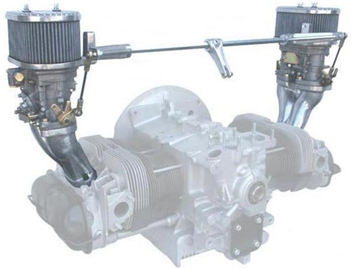
will be higher or lower. If it's higher, the second carburettor you are measuring is allowing MORE air into the engine than the first one is, and if it's lower, the opposite is true.
