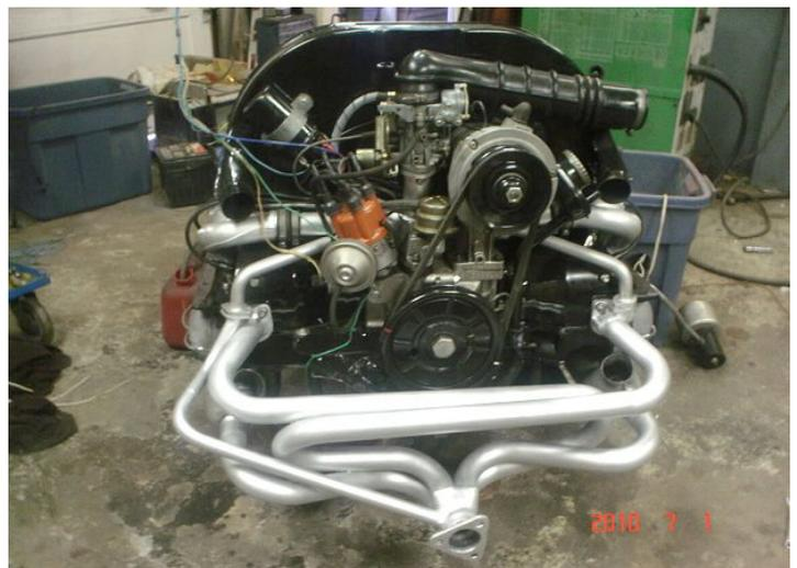
If you run a centre-mounted carb on a horizontally-opposed engine you need supplemental heat to insure proper vaporization in the runners. No mystery to any of this, it's in all the books and has been for seventy years.
