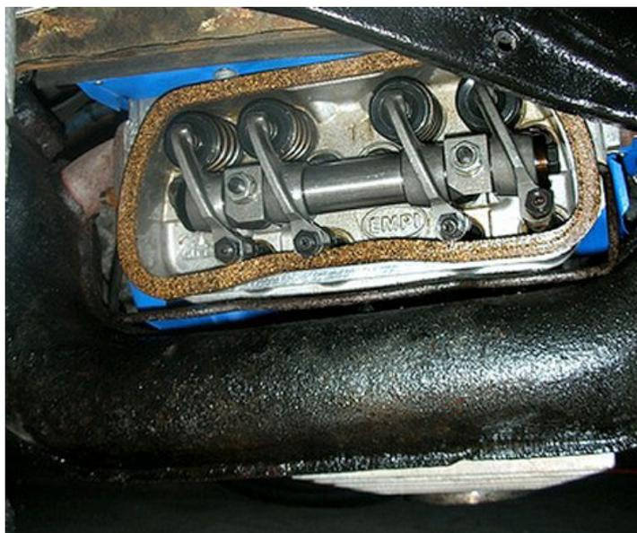
The less obvious reason has to do with the sealing surface around the valve gallery — the head surface against which the gasket is pressed to form the seal. If this surface becomes scratched or dinged — even slightly — it will not form an oil-tight seal. These scratches and dings usually occur when we adjust the valves.
