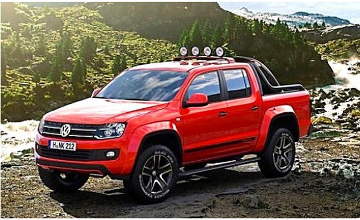
Adding to the Canyon's go-anywhere ability are roof-mounted auxiliary headlights, colour-contrasting under-body protection, 35 mm-wider wheel housings, and electrically deployed tread plates to help passengers step in and out.
