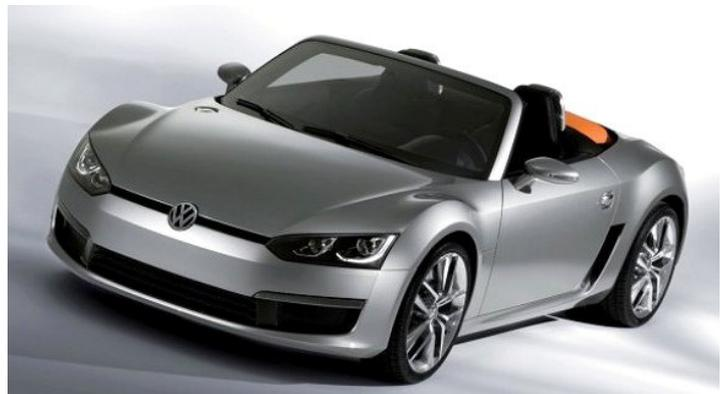
The 2009 Volkswagen BlueSport concept was just under four metres in length and powered by a 132 kW turbo diesel engine mounted in the rear, behind the two front seats. It was to be the first mid-engined VW since the VW-Porsche 914 of the early 1970s.
