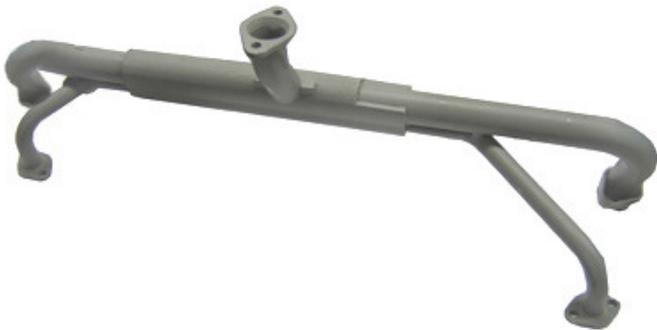
The pressure differential is important because the hot exhaust gases give up their heat to the centre section of the intake manifold casting (ie, where petrol absorbs the heat and changes its state from an atomized liquid to a true vapour). Once the exhaust gases have given up most of their heat, you must have that pressure differential to insure adequate gas-flow through the pipe.
