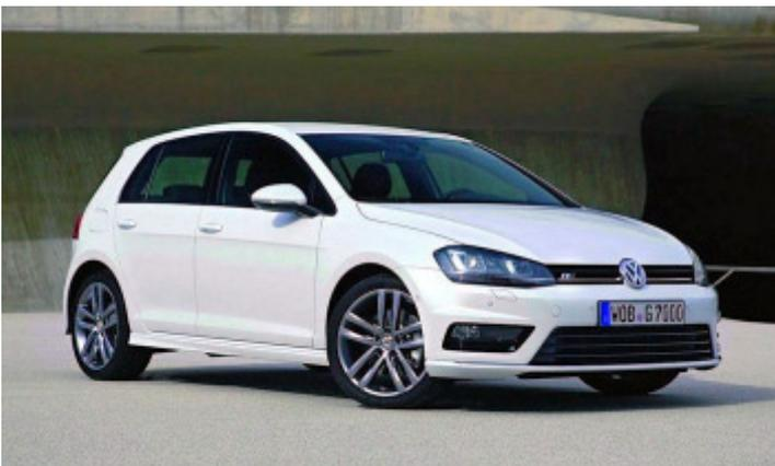
Exterior changes includes sports suspension (lowered by 15mm), 'Progressive Steering' that alters the steering ratio based on driver inputs, 18-inch alloys, front bumper extension and larger lower air intake, widened side sills, sportier rear bumper with black diffuser, a rear roof spoiler, tinted rear glass and R-Line badges.
