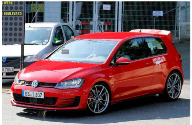
The car spotted at the infamous test track appears to be a Golf GTI Performance Pack with a range of changes such as 18-inch alloy wheels, larger red GTI-stamped brake callipers and lowered suspension, a half-size roll cage, a more pronounced front lip spoiler and an enormous roof-top spoiler.
