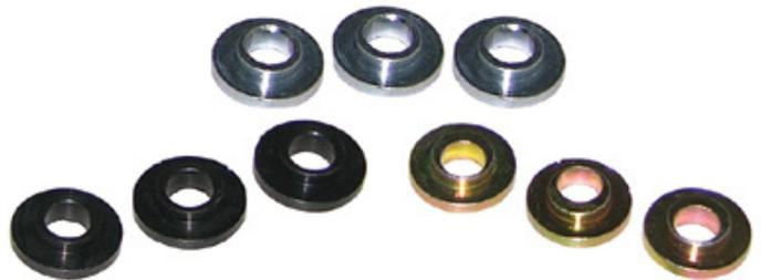
If you make up the washer so the pilot - the stepped portion -- is concentric to the bolt hole, your cam will be indexed straight up, without advance or retard. You may then install the cam and clock it. If clocking the cam sez you need to move it two degrees, you go over to the lathe and make up three new buttons with the hole offset by forty thou. That may sound like a major chore but trust me here, making eccentric buttons is a trivial task, assuming you have access to a lathe
