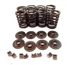
The strength of the stock VW valve spring is determined by measuring the amount of force needed to compress the spring to a height of 31.0 mm. A number of factors can affect the strength of a coil spring, and like all other VW specs, the tolerance is quite large, ranging from 53 to 62 kg force (520 to 610 Newtons, to be precise).
