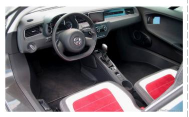
There's a simple instrument binnacle from the VW Up in front of the driver, a selection of Polo/Up switches on the centre console and a Garmin unit giving sat-nav, engine and fuel economy information. Two six footers will fit comfortably, with 120 litres of luggage space under the boot behind the engine.
