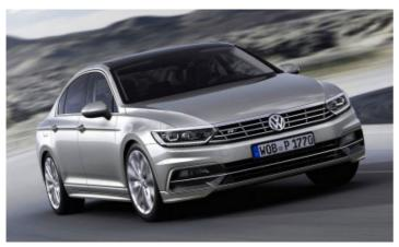
The B8 Passat is an all-new model based on Volkswagen's flexible MQB architecture. The new car weighs up to 85 kg less than its forebear and is said to be around 20 per cent more fuel efficient.
