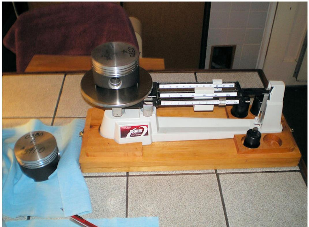
In the final stages, each time you weigh the piston you must make sure it is clean. The residue of metal you're removed will try to cling to the piston. It will get into the ring grooves and wrist-pin trunnions. And when it does, its weight will still be there.
