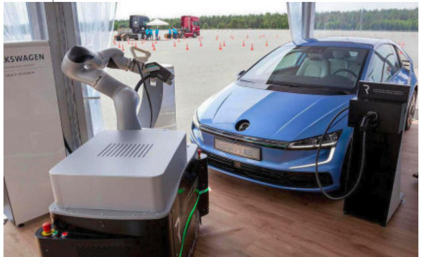
Most interestingly, the Gen.E can be recharged via a specially designed robot, which VW is developing to work in underground and multi-storey car parks to help automatically connect electric vehicles up for recharging.
