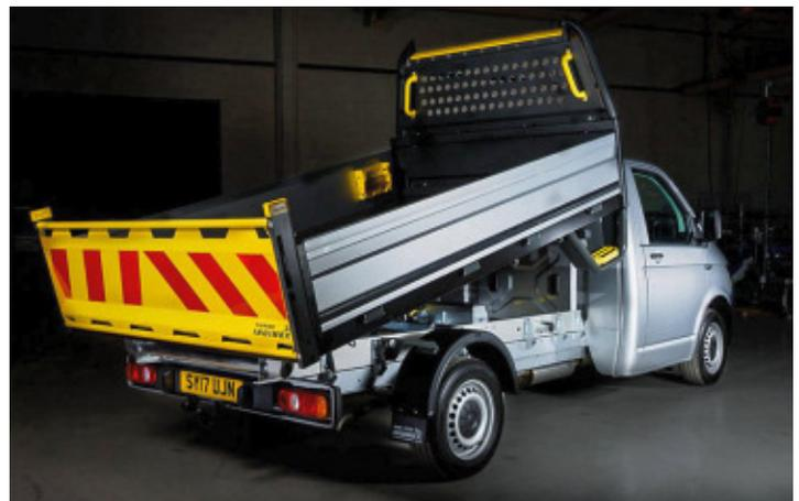
Created and developed in partnership with Volkswagen Commercial Vehicles (UK) by Ingimex Ltd – the UK’s largest manufacturer of light commercial vehicle bodies – the tipper body conversion is available for both T30 (3000kg GVW) and T32 (3200kg GVW) versions of the Volkswagen Transporter, offering payloads of around 800 kg and 1000 kg, respectively.
