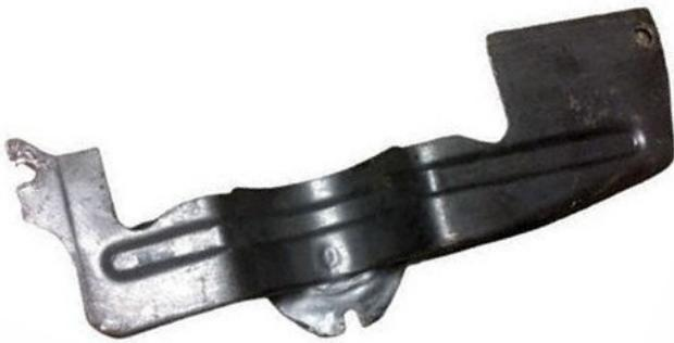
o What does this piece of tinware even do? It was used in the late 60s and fits around the crankshaft pulley. I keep telling anyone who cares to listen "VW knows best - don't leave off any parts or the engine will overheat", but not in this case, and even VW saw fit to scrap it.
