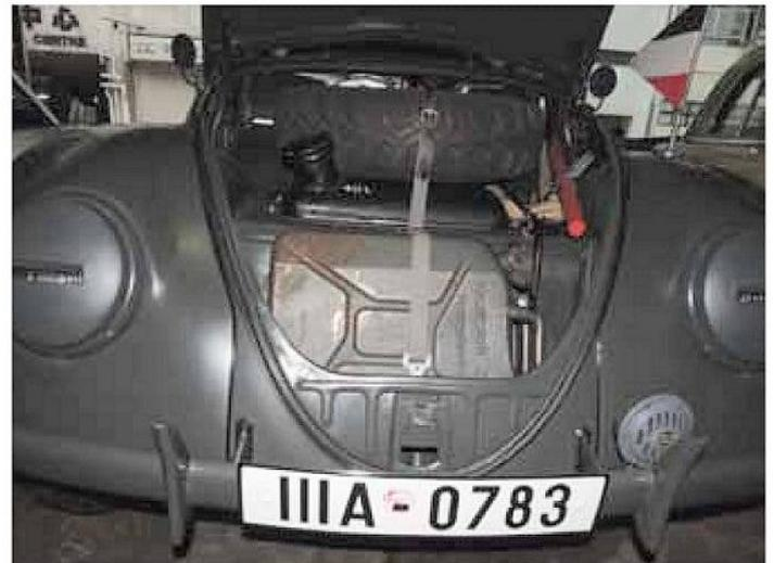
*Like a normal wartime Beetle, the 1941 Type 877 prototype carried a spare tire, 20-liter fuel gas can, rear air filter and twin puller set under the front hood. These items are all original to Victor's vehicle.*
