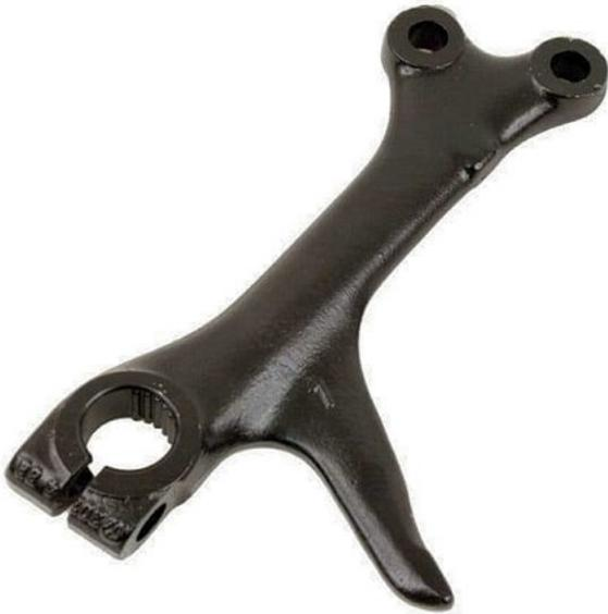
o Would someone please explain to me why the hole where the short tie rod fits on the Pitman arm is further outboard than the one where the long one goes? Is it the only way to maintain proper Ackermann geometry with an offset steering box? I have never seen or heard an explanation.
