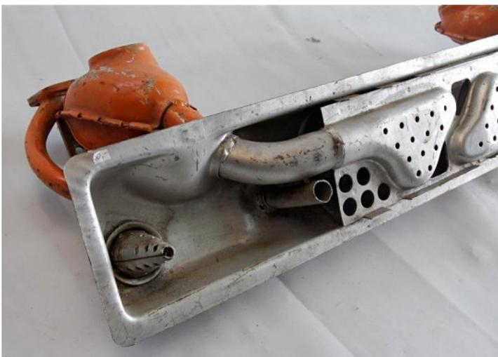
up and muffling stayed the same. On the other hand, hot gas impinging on the walls of the tin box may shorten its life, but they could have used a double panel in those spots. I'm just as baffled as the muffler.
