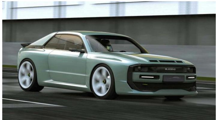
E-Legend claim range of up to 400 km for the EL1, but confusingly, they also say the battery allows for only two flat-out laps of the 20.83 km Nurburgring Nordschliefe - that's only 10 per cent of the claimed maximum range. Obviously the range shrinks considerably when you use the power available to its maximum.
