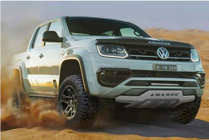
As with the road-focused VW Amarok W580S, there will be no extra power or torque planned for the turbo diesel 3.0-litre V6. But it is already the most powerful vehicle in its class with outputs of 190 kW/580 Nm (200 kW on overboost).
