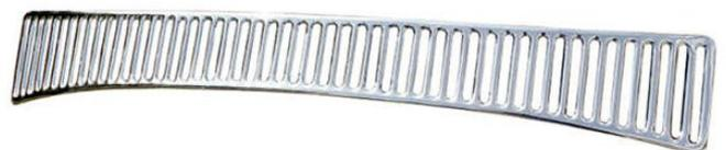
o I only recently found out that VW changed the number of slots in the cooling air intake from 50 to 42, for 1303 (Superbug) models only. Was this a stealthy way of packing more air in there? Part numbers 000 071 309 for the 50-slot version and 000 071 309 A for 42.
