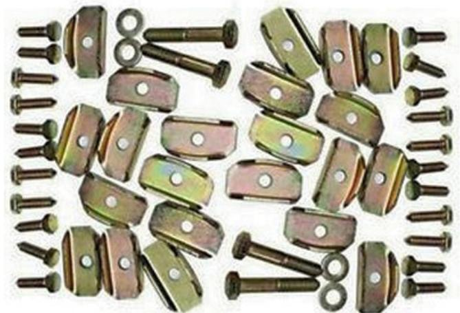
o Beetle body hold-down plates have a convex curve on one side and are straight on the other. Somebody designed the plate that way and then VW made them for years with that particular shape. Um, why? Is the orientation for assembly specified?
