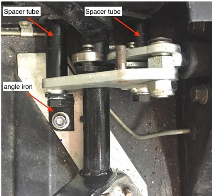
I figured that adding a simple bracket made of angle iron to brace the assembly to the floor plate would help tie it in to existing structures. This thing is a goer! The stock pushrod is replaced with a shorter one which still has an adjustment for the all-important free play. A spring, missing in the pic above, eliminates play between the bearing and the cam. It will be a while before I can confirm that braking effort is reduced by 35%, however.
