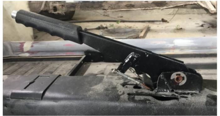
A triangular piece has been welded back in to the bracket to improve support. Notice that the pivot point for the cables on this Golf-1 handbrake is underneath? E-clips are much easier to work with than those silly wire circlips.
