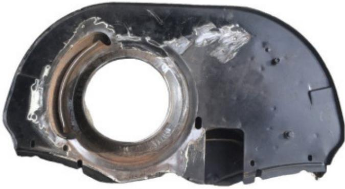
Fan housing after removal of stock oil-cooler exit panel
