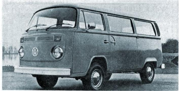
VW is now offering a bigger (1700cc) engine and automatic transmission in the 1973 range of commercial/passenger vehicles. The Kombi will now be available with 1600cc and 1700cc engine. The automatic is optional on the 1700cc model and is a T-bar shift mounted on a central console between the front bucket seats.
