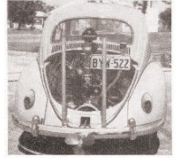
"SNORKEL" EXHAUSTS and propeller are fitted to the back.
