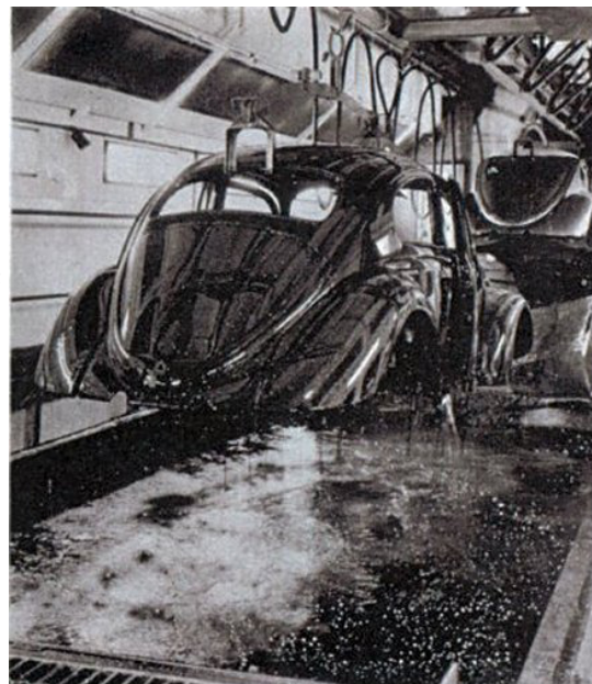
The "black dip" in which Volkswagen bodies are completely immersed to give complete protection of all sections. The tank holds 7,000 gallons of paint.
