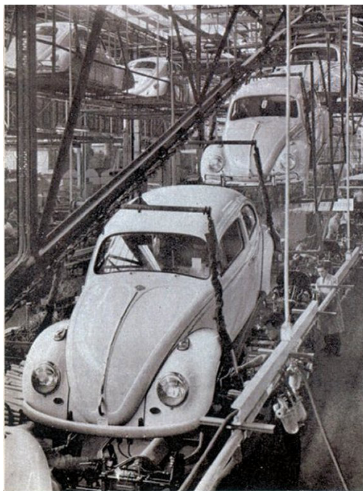
Volkswagen 1200 sedan bodies on the automatic body drop coming down to meet the chassis moving on the conveyor beneath them.
