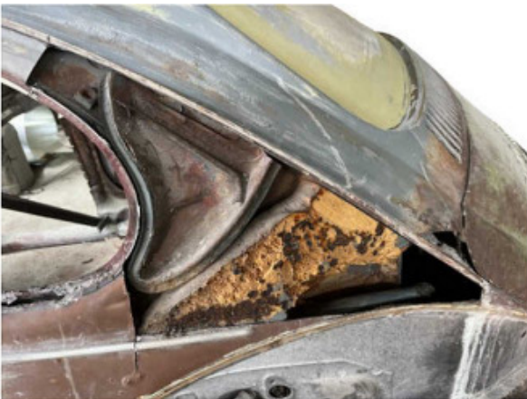
I cut this section of steel out so that you don't have to. Shown is the bedpan piece with baffle on top, before drilling out, and all that nasty foam. The hidden vents run level with the roof crimp.
