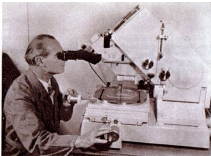
The accuracy and standardisation of the size, shape and form of tools is an essential part of automotive engineering. This Zeiss microscope, kept in a constant temperature room, measures the slightest variation from standard in a tool by optical means.
