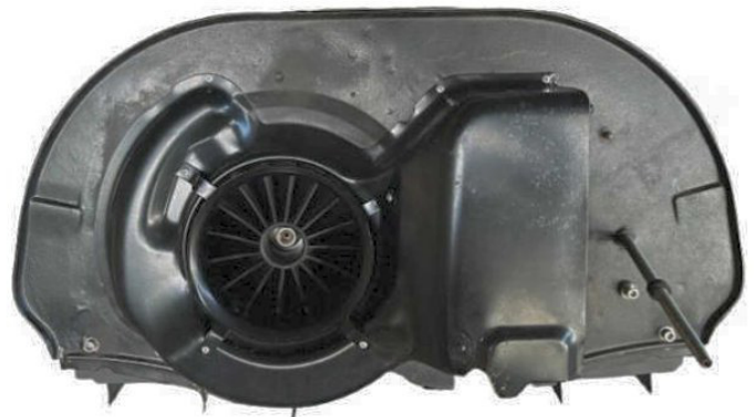
Black on black makes it hard to see, but the venturi ring is now in place. Also visible here: the Andrig plastic fan , Andrig's fixed flaps , the beautiful Concept 1 Type-4 oil-cooler tin and the relocated Bowden tube for the accelerator cable.
