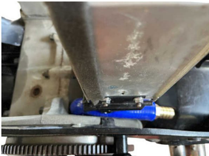
The hose is firmly held in place by the narrow crevice between the Hoover bit and the crankcase mating flange. It could not be a tighter fit than this.
