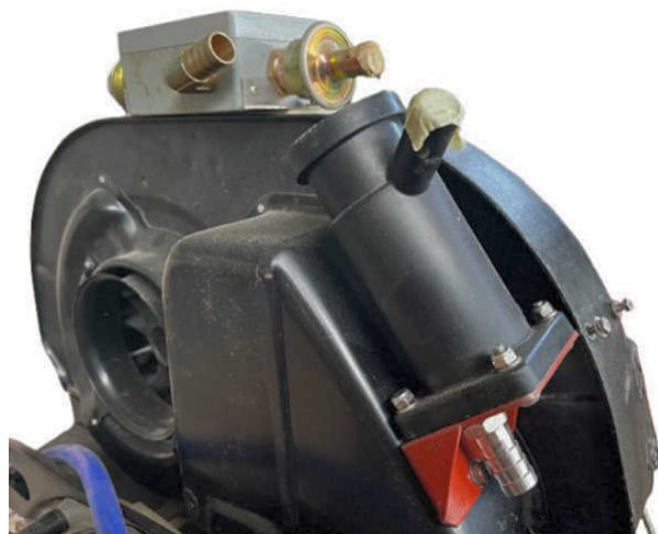
The T3 Transporter breather tower has a scouring pad inside. It will connect to one of the check valves screwed into the sealed box on top of the fan housing.
